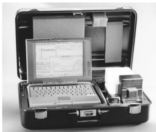
Fig. 1 Photograph of the briefcase-sized, rechargeable, battery operated, portable MATCI. Reproduced from ref. 11 with permission.
