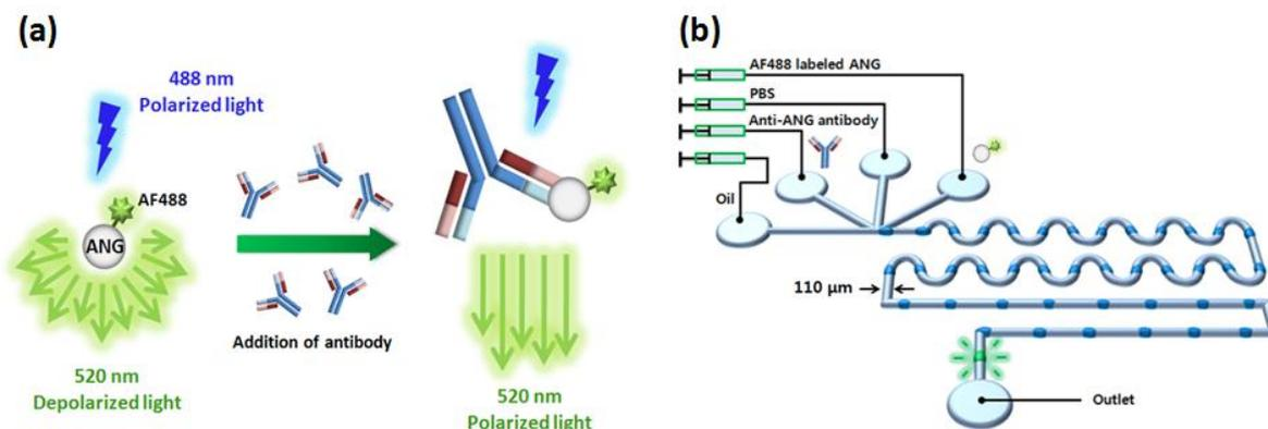
Figure 1. (a) Schematic of the fluorescence polarization facilitated by protein-protein interactions. (b) Layout of the microfluidic device for experiment. The AF 488 labeled angiogenin (ANG) solution is flowing into the right inlet, while anti-ANG antibody solution is flowing into the left inlet. The phosphate buffered saline (PBS, pH 7.4) is delivered into the middle inlet.
