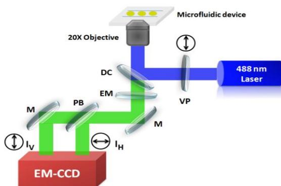
Figure 2. Schematic of the optical setup for fluorescence polarization measurements. The system consists of 488 nm laser for fluorophore excitation, 20X objective, dichroic mirror (DC), emission filter (EM), vertical polarizer (VP), adjust mirror (M), polarizing beam-splitter (PB), and electron multiplying-charge coupled device (EM-CCD).
