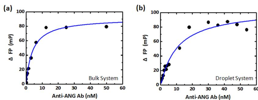
Figure 5. Analysis of interaction of angiogenin (ANG) with anti-angiogenin antibody (anti-ANG Ab) by fluorescence polarization. (a) In bulk system, the concentration of AF488-ANG was fixed at 1.25 nM, while the concentration of anti-ANG Ab varied 0 to 50 nM. (b) In droplet-based microfluidic system, the concentration of AF488-ANG was fixed at 5 nM, while the concentration of anti-ANG Ab varied 0 to 54 nM.
