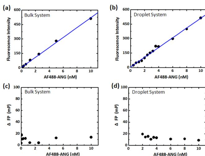
Figure 3. Fluorescence intensity (a, b) and polarization value (c, d) versus the concentration of the AF488-ANG in bulk fluorescence polarization system (a, c) and droplet-based microfluidic system (b, d).
